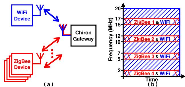
Figure 2: Our approach enables concurrent communications i) from commodity WiFi and ZigBee devices to the gateway; and ii) from the gateway to commodity WiFi and ZigBee devices. Therefore, the spectrum utilization is significantly increased.
