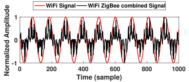
Figure 3: Combined WiFi and ZigBee Signals
