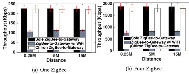
**Figure 13: Throughput of ZigBee-to-Gateway Link: When WiFi traffic exists, the throughput of Chiron ZigBee-to-Gateway is about 2.3 times higher than traditional gateway approach. Besides, Chiron ZigBee-to-Gateway is similar to sole ZigBee-to-Gateway which does not have WiFi traffic interference.**
