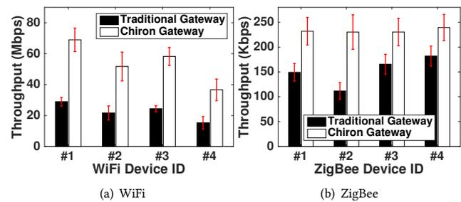
Figure 12: Multiple WiFi and ZigBee Devices Communicate with Chiron Gateway: Chiron gateway can concurrently communicate with four different ZigBee devices (which are on different ZigBee channels) while communicating with different WiFi devices alternatively.
