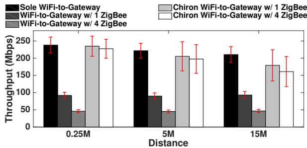
**Figure 16: Throughput of WiFi-to-Gateway Link:** Chiron shows similar throughput to sole WiFi-to-Gateway but almost 4 times of traditional gateway approach when four ZigBee devices exist.
