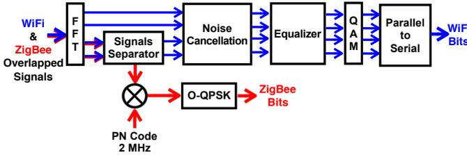
Figure 7: The Demodulation of Overlapped WiFi & ZigBee Signals
