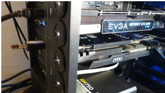
Simple Display Emulator with an HDMI-VGA Adapter
