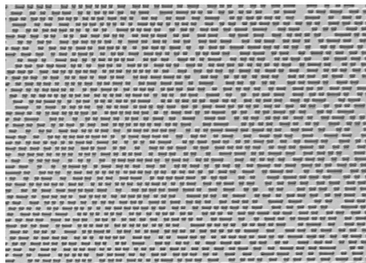
Close-up view of a CD surface, showing the pattern of pits and lands.
